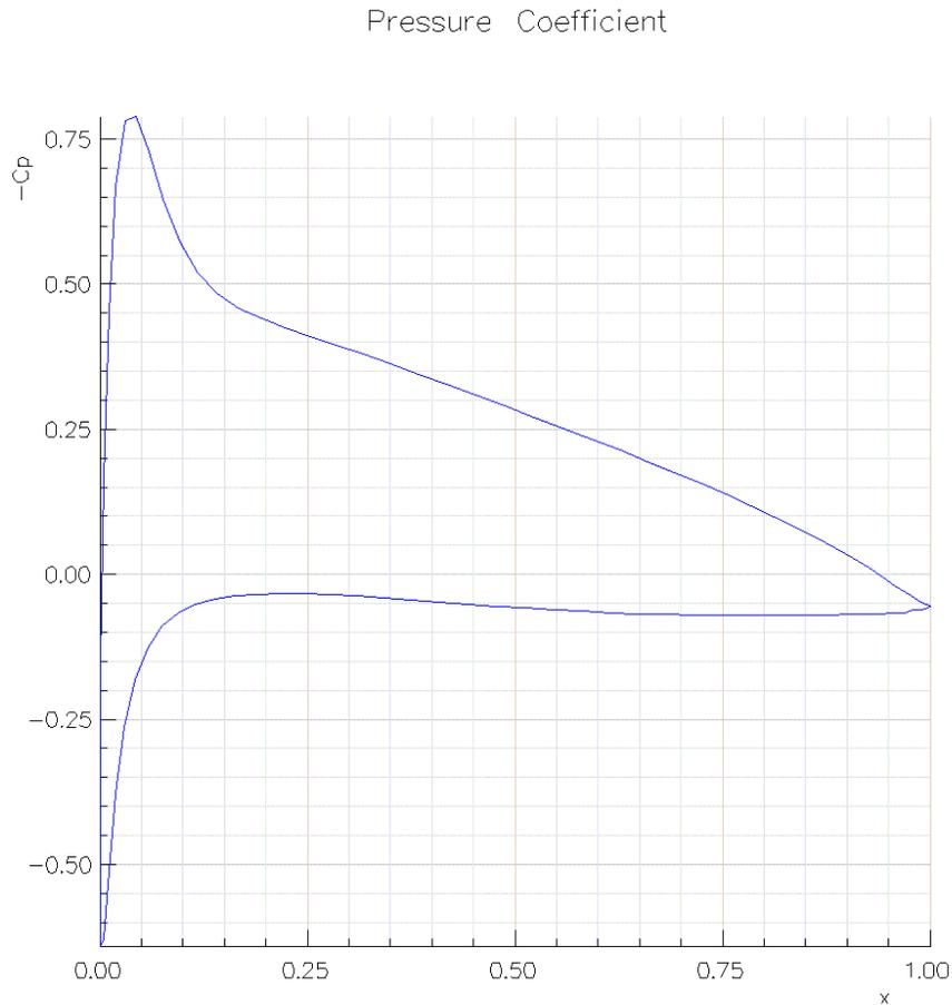
Figure 13: The `aero.C` program can be used to read a show file generated by `cgins` and compute the coefficient of pressure on the surface of a body.
