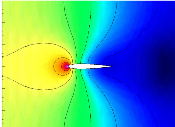
Figure 5: Incompressible flow past a NACA 0012 airfoil, pressure.
