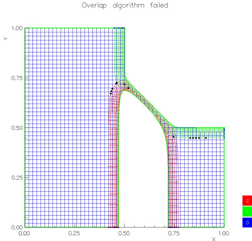
Figure 40: An example showing the failure of the overlapping grid algorithm when there is insufficient overlap. We have tried to use explicit interpolation for the two-dimensional valve. The algorithm fails and plots the offending points with black marks.
